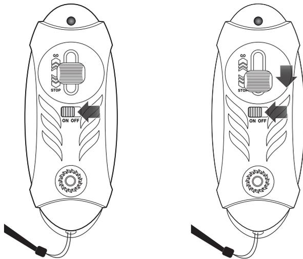
**1** While riding, release the remote lever and it will return to the "NEUTRAL" position. The product will slow to a stop with motor resistance.
