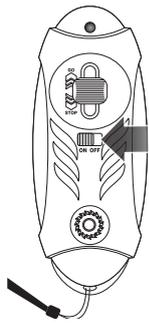
**1** Turn the power switch on the remote to the **ON** position.
