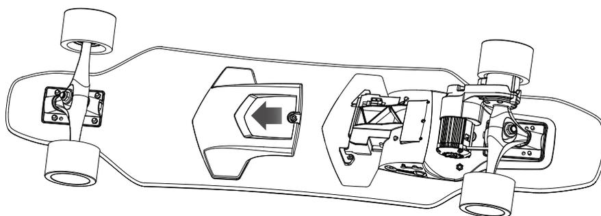
**2** Slide to remove the battery cover.
