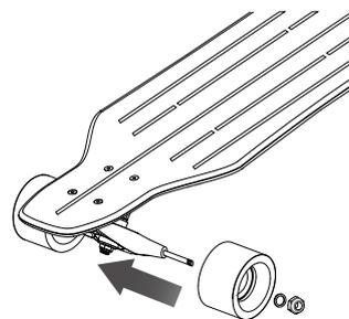
**3** Insert replacement wheel, washer and locknut.
