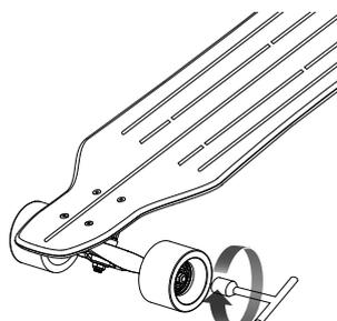
**4** Tighten the locknut.
