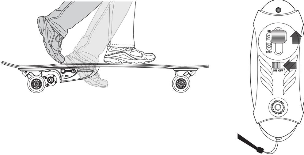
**Note:** RazorX Longboard Electric Skateboard must be moving at least 3 mph (5 km/h), with lever on remote in GO position, for motor to engage.
