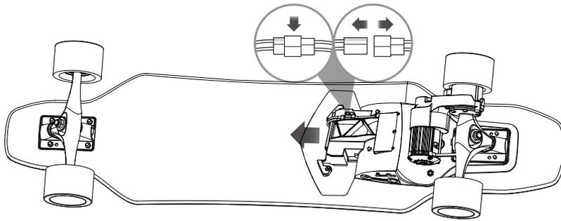
**3** Disconnect the battery connector from the control module and carefully remove battery.
