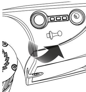
**2** Open the pairing button cover located underneath the power button.
