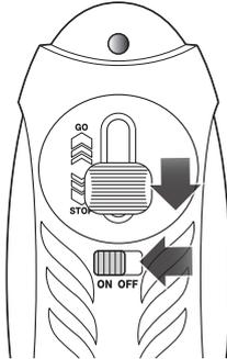
**4** Move the lever on the remote to the **"STOP"** position and **HOLD**. **Do not let go of the lever.** Turn the power switch on the remote to the **ON** position.
