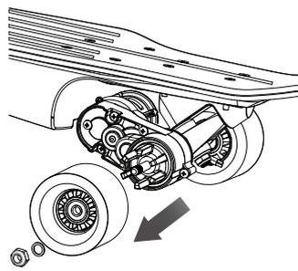
**2** Remove the locknut, washer and wheel.
