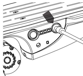
**2 Note:** Make sure power button is in the **OFF** position. Plug the charger into the charger port. The light on the charger should turn red during charging. The light will turn green again when charging is complete.
