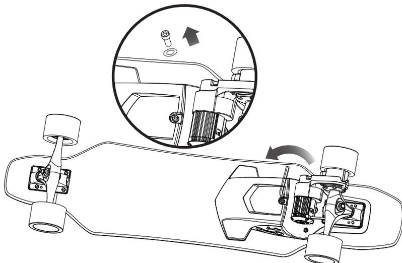
**1** Carefully turn product over. Loosen and remove the bolt and lock washer from battery cover.
