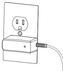
**1** Plug the charger plug into wall outlet. The light on the charger should be green.
