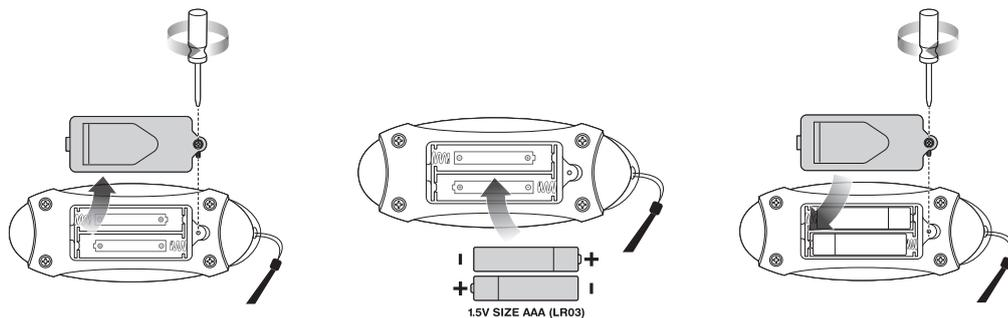
**1** Loosen Phillips screw on battery cover and remove cover. Remove old batteries and properly dispose.
