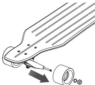
**2** Remove the locknut, washer and wheel.
