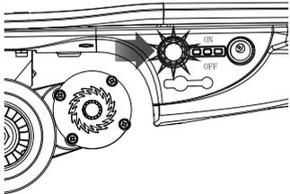
**6** If the light on the product continues to flash quickly, turn power switch on the remote to the **OFF** position and repeat steps 3-4 until remote is paired.
