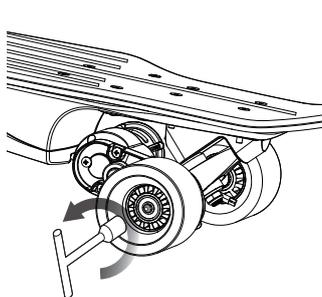
**1** Using the 13 mm socket, loosen the locknut.
