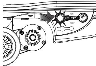
**3** If power button on product is **flashing**, leave power button on the product in the **ON** position. See Pairing the Remote section below for pairing instructions.
