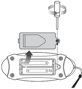
**1** Loosen Phillips screw on battery cover and remove cover.
