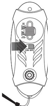
**1** Turn the power switch on the remote to the **OFF** position.
