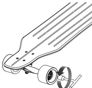
**1** Using the 13 mm socket loosen the locknut.
